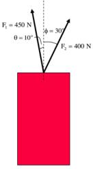
4.19) A 150-N potted plant is suspended by three cables as shown. What's the tension in each cable?
